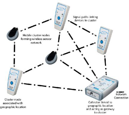
The system comprises a number of cluster node devices which communicate with one another using licence-exempt 2.45 GHz radio signals to form an adhoc mesh network. They use true radio range measurements to precisely determine how far they are from their neighbours in the network. Using the measured ranges the Omnisense Location Engine computes relative positions for all the devices in the network to high precision (1 to 3 metres) without needing any permanent or pre-installed infrastructure.
